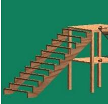
2- 2 x 6 10 feet long, horizontal flat ladder ramp rails, installs at six foot height
